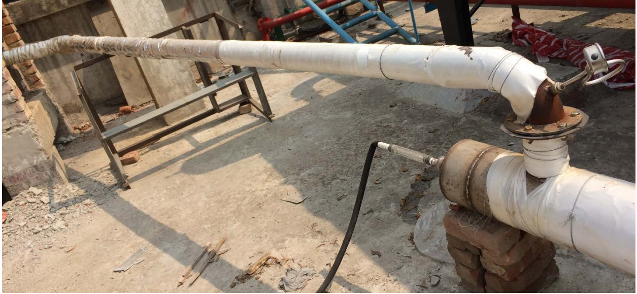
Figure 4.8: Water and Exhaust gas Inlet Set up.
