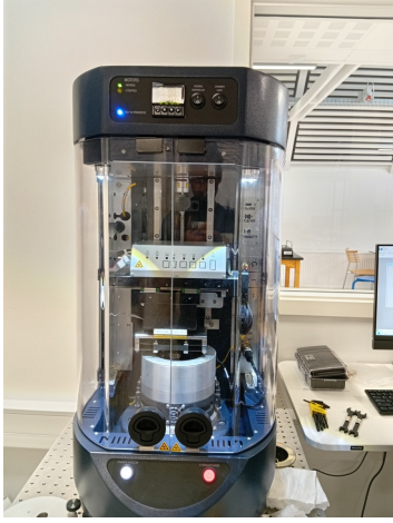
(a) Bruker UMT TriboLab setup (Front)
